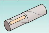
Hold your telescope with the inner tube facing your eye. Aim it at an object in the night sky. (Never use your telescope to look at the sun!) You can focus by sliding the inner tube in and out.
